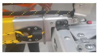
Secure with Nuts: Wind the nuts onto the U-bolt and tighten them using torque wrench 9Nm to secure the bracket in place.
