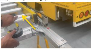
Align the Bracket: Position the bracket on the stile connector of the ladder so that it wraps around and envelops the TerrainMaster.
