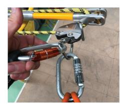
Disconnect the front chest attachment from the rope grab device so only the lanyard is attached.
