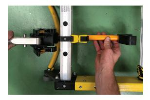
Press down on the black latches to lock the Davit accessory to the ladder top attachment.
