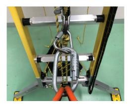
Tension the rope line by lower the users weight until the ladder is supporting the users load via the rope line.
