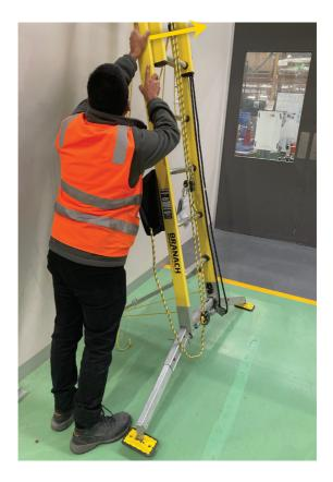
Fit an approved harness and appropriate PPE and connect the front chest-D to the Fall Control rope grab.
