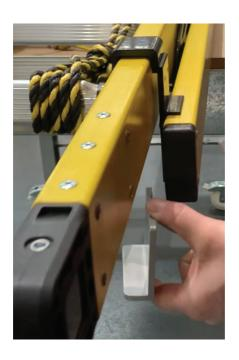
Fit the backing plate around the black top guide bracket.
