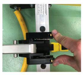
• Check both latches are fully closed and the gold locks are level with the black latch surface.
