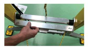
Fit the T-bar into the cross bar until it locks into position, capturing the rung. You may need to loosen the tethers to do this.
