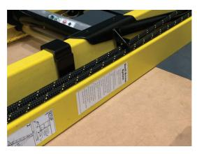
Between the Davit Access System label and the Fall Control setup diagram, place the "Davit Ready" label.
