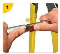
To open the latch, slide to the left and separate.
