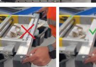
Align the bolt pin to the stile connector.
